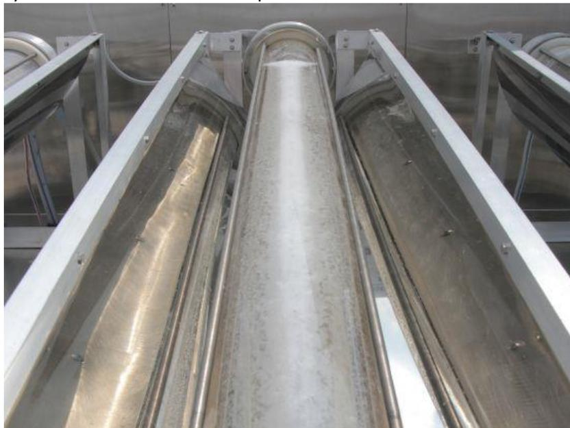
One of the reactor tubes of the hydrogen-generation system shows fine bubbles of hydrogen gas rising to the surface of the water. Photo: Zara Zhuang
